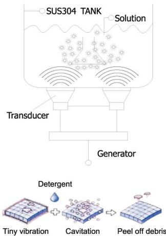
Ultrasonic cleaning is extremely effective at removing dirt and grime which would normally require tedious manual cleaning by hand. It has been used to clean a wide variety of instruments and mechanical parts such as carburetors, returning them to almost like new condition without damage to delicate parts.
